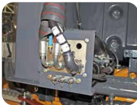
Easily accessible test ports allow technicians to troubleshoot problems more quickly.
