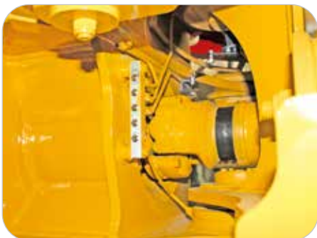
The centralized lube bank places difficult-to-reach grease points within reach.
