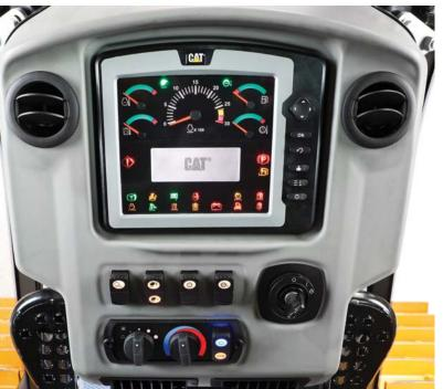
All controls are electro-hydraulic, which means precision and maneuverability. They are ergonomically designed for easy intuitive, comfortable and low effort operation. Blade response can be adjusted through the operator profile in the display.
