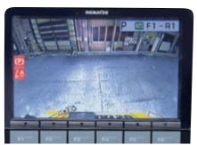
Fully integrated rear-view camera system
