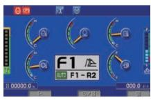
Automatic gearshift mode to further reduce fuel consumption
