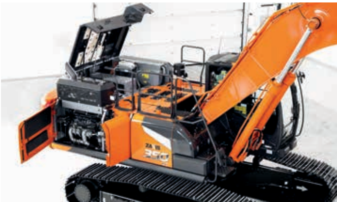
Engine cover with dampers (ZX300/ZX350) enables convenient access for daily inspections.
