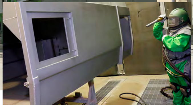
Shot blasting the hopper's stainless steel body
