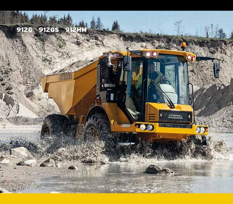
A unique combination of articulated center pivot, wide tyres and high ground clearance - for superior off-road performance.
