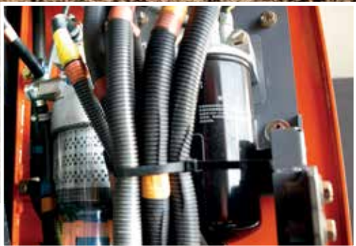
The main fuel filter is easier to replace.
